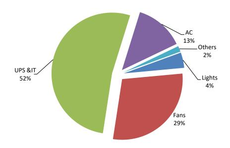
Fans account for 29% of the overall energy consumption in this facility, while lighting utilizes 4%, UPS and IT contribute 52%, and other miscellaneous uses constitute 2%. Additionally, 13% of the total energy is consumed by air conditioning systems.
